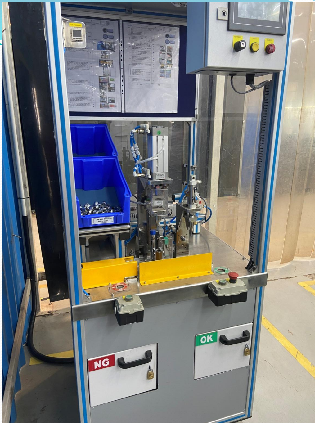
Cable Ball Socket Cap Load Check and Auto Greasing
